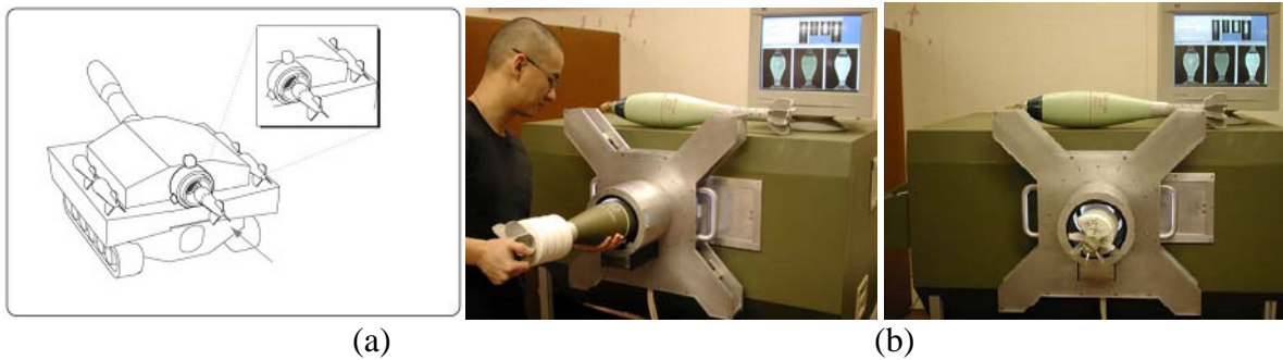
Figure 13. (a) Concept future force mortar with PIDS system inline with loading port. (b) PIDS ID and inspect system as implemented for port inline application.
