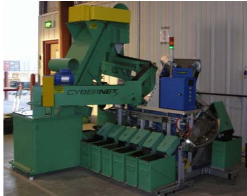
Figure 12. (a) Bulk turn-in ammunition (b) ATACS bulk ammunition inspect and sort
