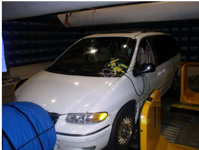
Figure 22. The Grand Challenge Vehicle under test at the General Motors Electromagnetic Test Facility for determination of microwave weapon assault susceptibility (projects for the Dept. of Homeland Security and TSWG)
