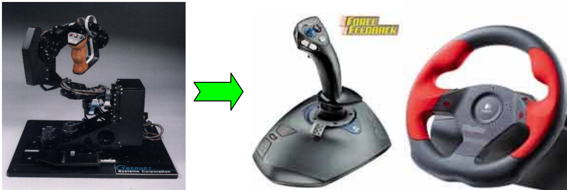
Figure 1. Cybernet force feedback device built form NASA (left); Commercial derivatives licensed by Immersion for Cybernet (Right – Logitech products)
