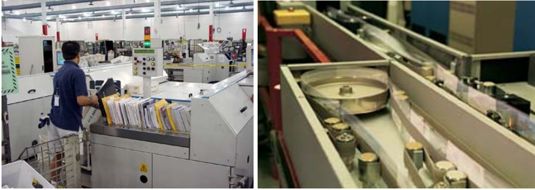
Figure 17. USPS letter and flats sorting machines using handwritten and machine print OCR automation developed by Cybernet/NetMAX staff while they worked at the Environmental Research Institute of Michigan, 1987-1990.
